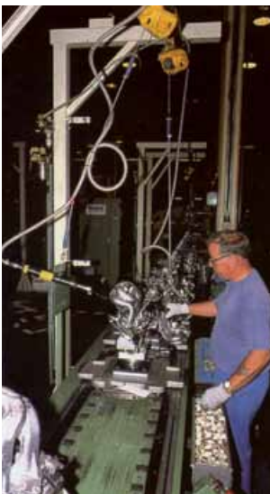
Suspended hand tool in use, showing support cable
