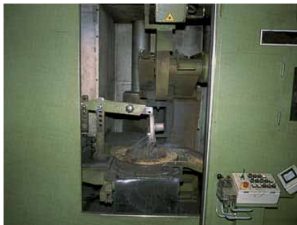
Automatic cut-off machine showing a casting in a fixture
