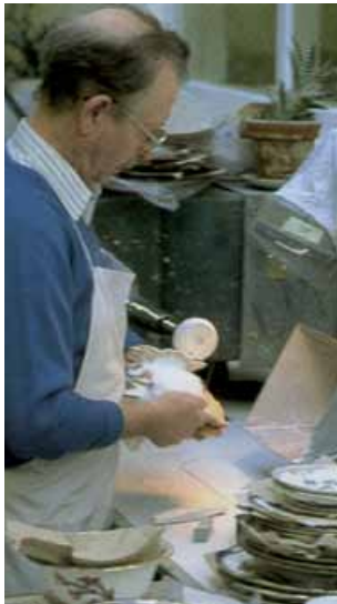
Ware being polished with a pedestal machine
