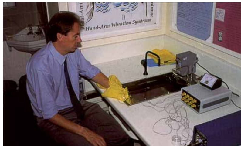
Hand in 15°C water tank for cold provocation test
