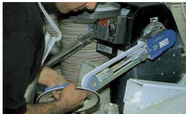
Ware being polished with a bench-top linisher machine
