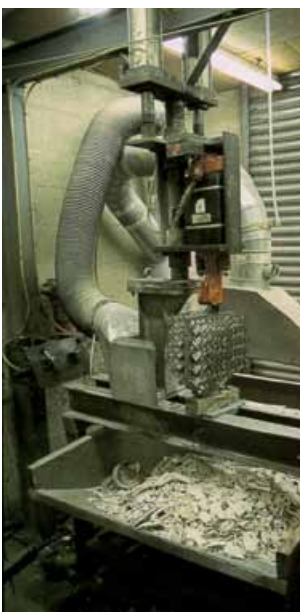
Knockout machine showing breaker mounted in support frame
